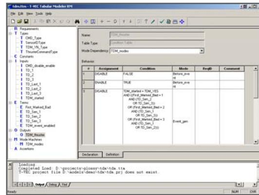
T-VEC Tabular Modeler (TTM) captures and manages precisely defined requirements that are then used to automatically generate tests.
