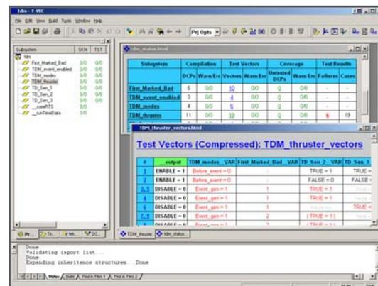
T-VEC Graphical Environment provides an interface to generate and view test vectors, test drivers, reports and status.
